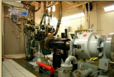
This cylinder head is equipped with Sturman digital hydraulic valve actuation.
