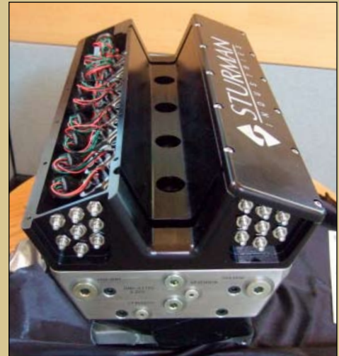
This cylinder head is equipped with Sturman digital hydraulic valve actuation.
